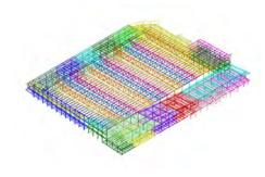
GRAEF is also using Autodesk® BIM 360® coordination tools to bring its steel detailing in Advance Steel together with the Revit model to help the firm collaborate with architects. "We can overlay the Advance Steel model over our Revit model and shoot a section over to the architects" explains Vogel. The same coordinated model can then be used to automate shop drawing production as designs evolve, helping to cut down timelines.
